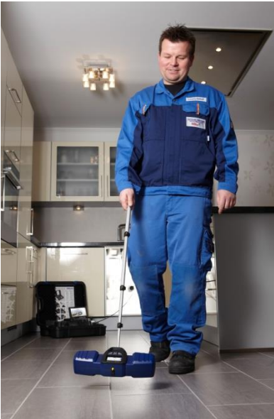
Fig. 13: Localizing the camera head underground
