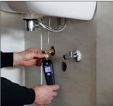
Fig. 5: Connection with angle adapter 90° (art. no. 8841)
