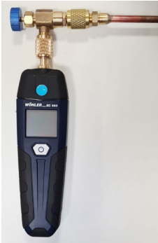
Fig. 12: Wöhler SC 660 connected to refrigeration system
